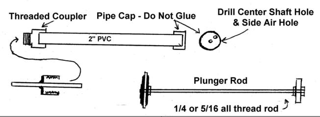
Female coupler with a  $2 - \frac{1}{2}$ " Reducer in the end. The reducer Will need to be reamed slightly To slide the  $\frac{1}{2}$ " PVC through. The  $\frac{1}{2}$ " PVC is at least 12" long and centered.
